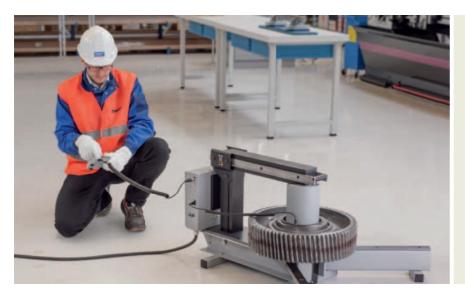
The TIH L MB induction heater is equipped with a remote control panel for operator safety.
