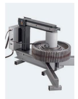
The TIH L MB heats non-bearing workpieces up to 600 kg (1 323 lb), depending on the model.
